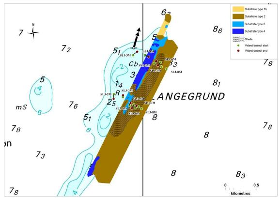
Figure 22. Sidescan interpretation results of Langegrund showing the DSC ground truth transects together with the substrates of the area.
