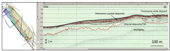
Figure 32. Innomar seismic section showing the Holocene coastal deposits, the glacial deposits and some possible Holocene slide deposits.
