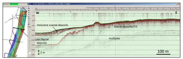
Figure 25. Innomar seismic section showing the Holocene coastal deposits, the late glacial deposits and the glacial deposits on a cross line.
