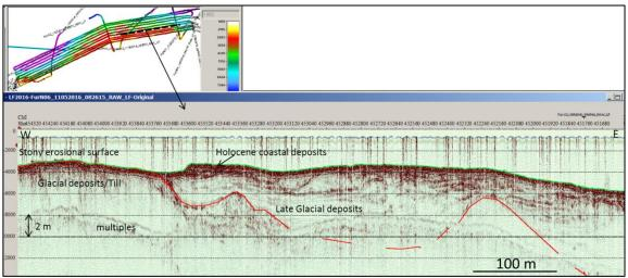
Figure 14. Innomar seismic section showing the Holocene coastal deposits, the late glacial deposits and the glacial deposits giving rise to the stony seabed surface.
