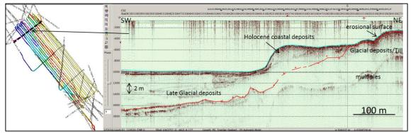
Figure 31. Innomar seismic section showing the Holocene coastal deposits, the late glacial deposits, the glacial deposits and the erosional surface in the northeastern end of the profile showed on a cross line.
