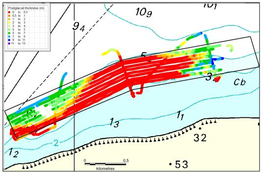
Figure 16. The thickness in m of the postglacial deposits or the depth below the sea bed to the glacial surface.
