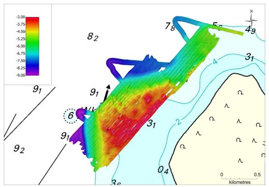
Figure 12. Livø North bathymetry. Legend represents depths in meters.
