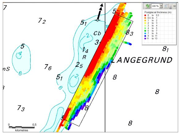
Figure 21. The thickness in m of the postglacial deposits or the depth below the sea bed to the glacial surface.
