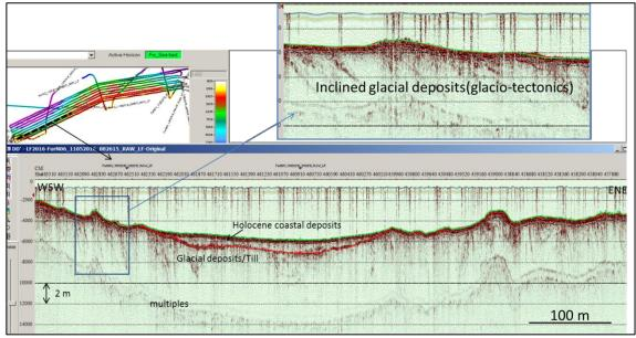
Figure 15. Innomar seismic section showing the Holocene coastal deposits and the glacial deposits revealing eastward inclined surfaces interpreted as glacio-tectonic thrust surfaces.
