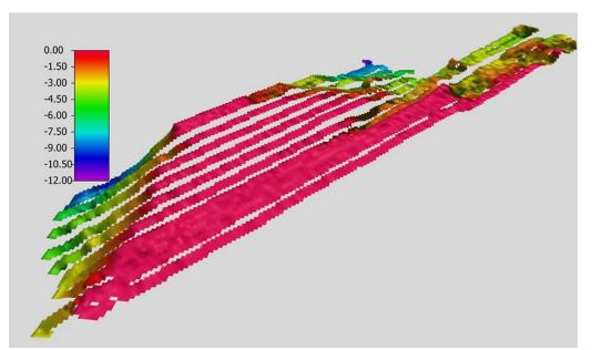
Figure 38. A 3D morphology of the topglacial (till) layer in Livø North. Legend values are depths below seabed in meters.
