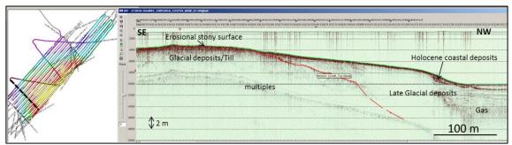
Figure 9. Innomar seismic section showing the Holocene coastal deposits, the late glacial deposits and the glacial deposits on a cross line.
