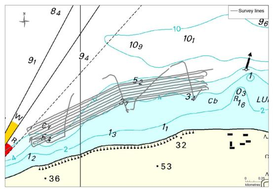
Figure 13. Fur North survey lines. The line spacing is 25-40m.
