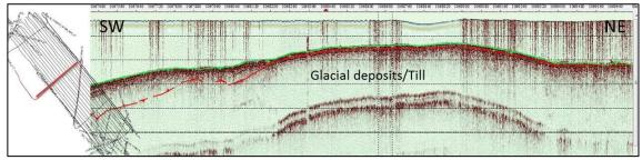
Figure 51. Livø Tap (South) seismic section perpendicular to the coast showing the postglacial layer thickness.
