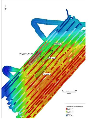
Figure 42. New stone reef positions in Livø North. Polygon named "Polygon 1\_GEUS" is the new position that replaces the previously suggested "Polygon 1" position.
