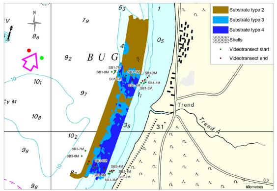
Figure 28. Sidescan interpretation results of Bjørnsholm showing the DSC ground truth transects together with the substrates of the area.
