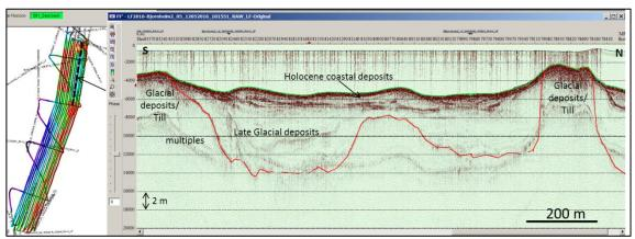
Figure 26. Innomar seismic section showing the Holocene coastal deposits, the late glacial deposits and the glacial deposits.
