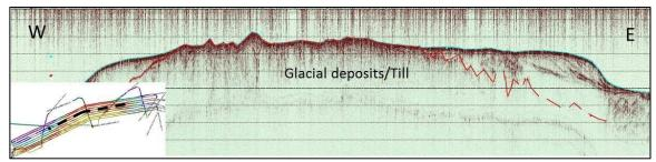
Figure 43. Seismic profile in Fur North showing the topglacial layer (till) exposed at the seabed.
