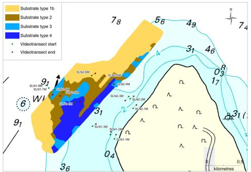
Figure 11. Sidescan interpretation results of Livø North showing the DSC ground truth transects proposed by GEUS.
