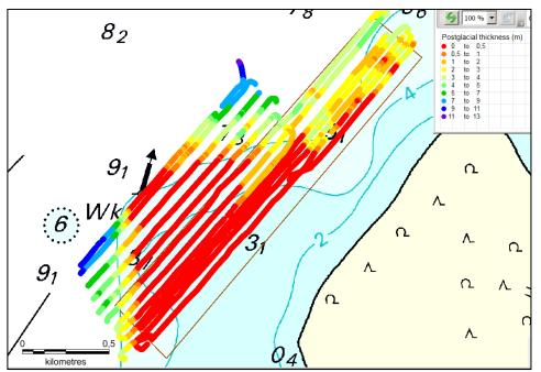
Figure 10. The thickness in m of the postglacial deposits or the depth below the sea bed to the glacial surface.
