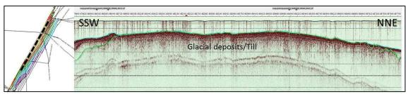
Figure 46. Seismic profile from Langegrund showing the glacial deposits (till) exposed at the seabed.
