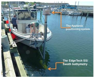
Figure 6. The Applanix positioning system configuration.
