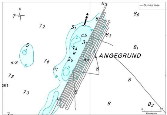
Figure 19. Langegrund survey lines. The line spacing is 25-40m.
