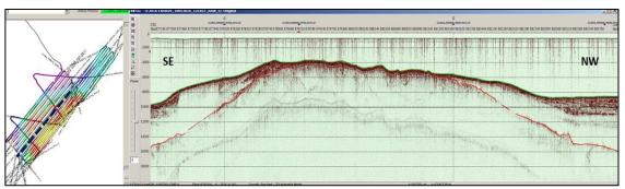
Figure 39. Seismic profile SE-NW showing the glacial layer (till) rising until it reaches the seabed in the centre of the profile.
