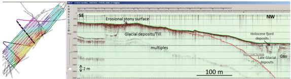
Figure 7. Seismic profile interpretation of a cross line shown in black on the left. Red line in the seismic profile is the top glacial surface.
