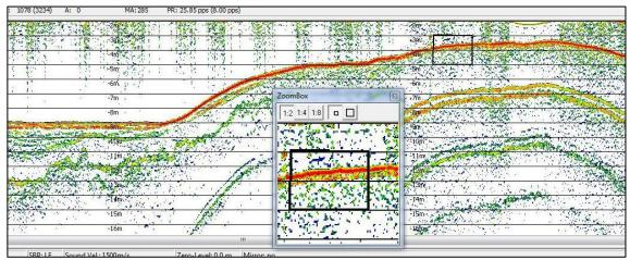
Figure 54. Livø Tap showing a zoom in high resolution image of the top section of the seismic profile (same as in Figure 51). It shows a thin second layer overlaying the glacial till.
