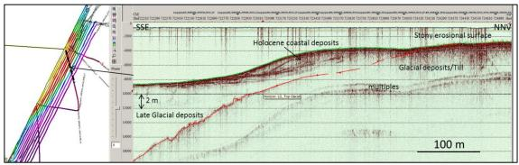
Figure 20. Innomar seismic section showing the Holocene coastal deposits, the late glacial deposits and the glacial deposits giving rise to the stony seabed surface.
